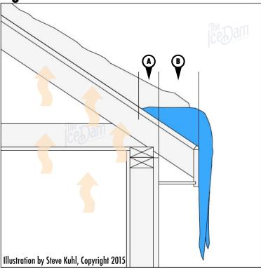
Figure 2: Ice Dam With Guttters
